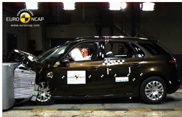
Frontal offset test at 64 km/h (Euro NCAP test of C4 Picasso)
