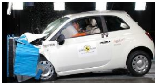
Offset crash test at 64km/hr
