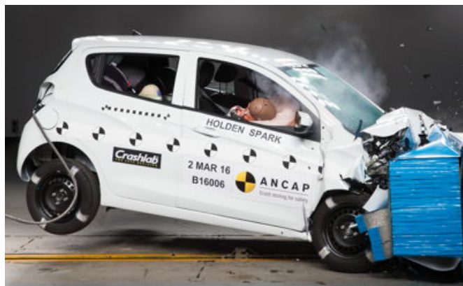
Frontal offset test at 64km/h
