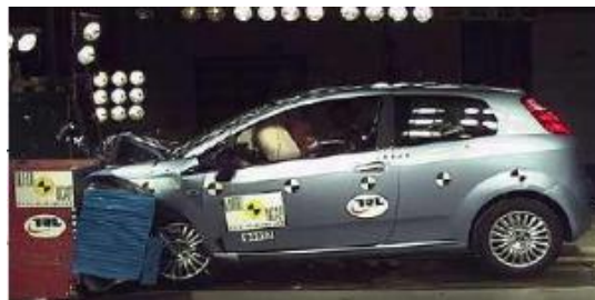
Offset crash test at 64km/hr
