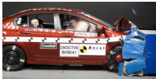
Offset crash test at 64km/hr
