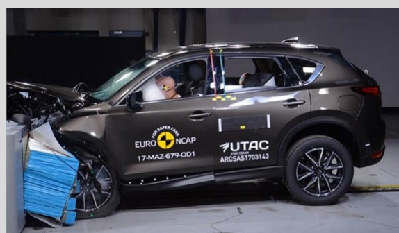
Frontal offset test at 64km/h
