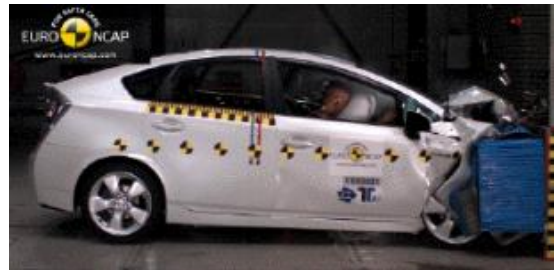
Offset crash test at 64km/hr
