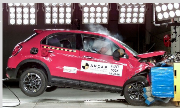
Frontal offset test at 64km/h
