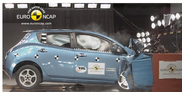
Offset crash test at 64km/h
