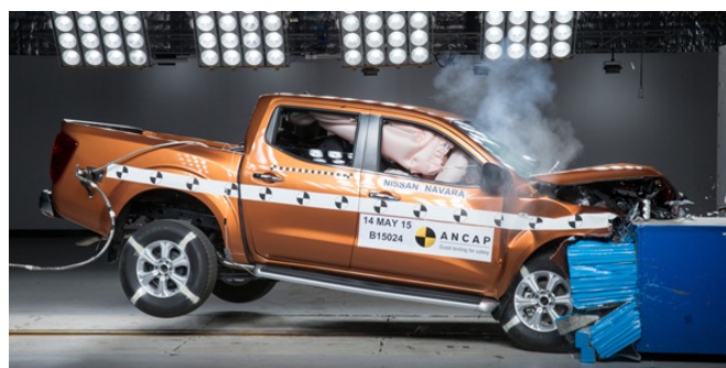
Frontal offset test at 64km/h
