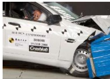
Offset crash test at 64km/hr
