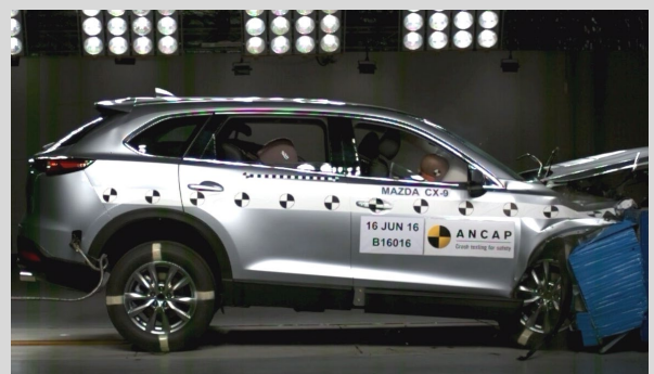
Frontal offset test at 64km/h
