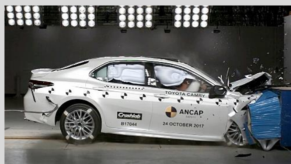
Frontal offset test at 64km/h
