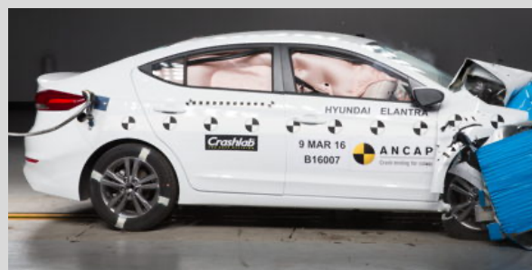
Frontal offset test at 64km/h (Hyundai Elantra)
