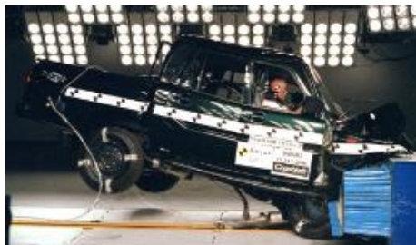
Offset crash test at 64km/hr
