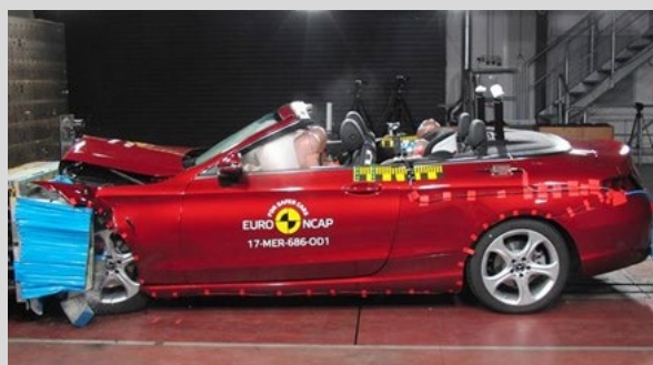
Frontal offset test at 64km/h
