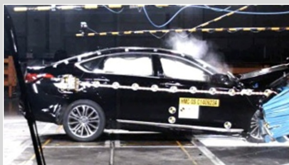
Frontal offset test at 64km/h
