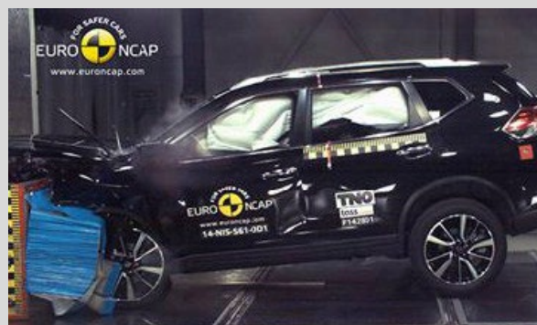
Frontal offset test at 64km/h
