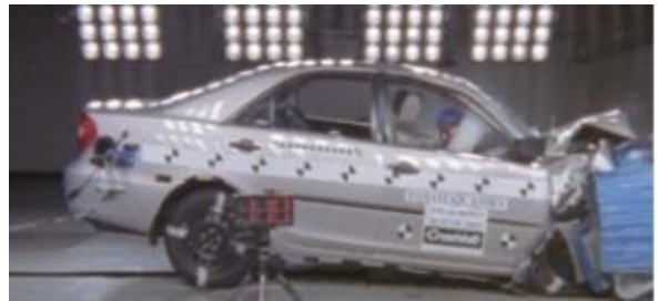
Offset crash test at 64km/hr
