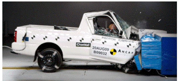
Offset crash test at 64km/h
