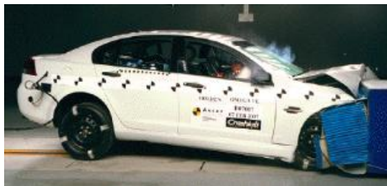
Offset crash test at 64km/hr
