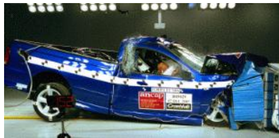
Offset crash test at 64km/hr
