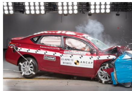
Frontal offset test at 64 km/h
