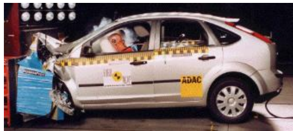
Offset crash test at 64km/hr
