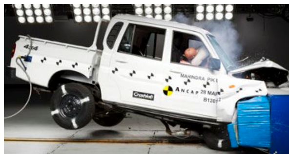
Offset crash test at 64km/h
