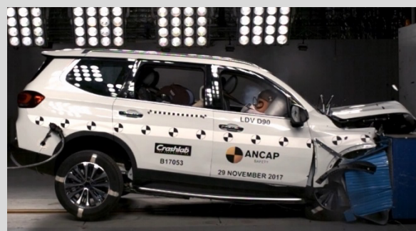
Frontal offset test at 64km/h
