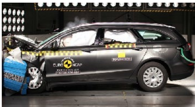
Frontal offset test at 64km/h (Euro NCAP - wagon)
