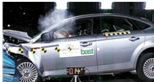
Offset crash test at 64km/hr
