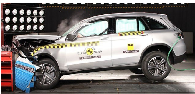
Frontal offset test at 64km/h (Euro NCAP)
