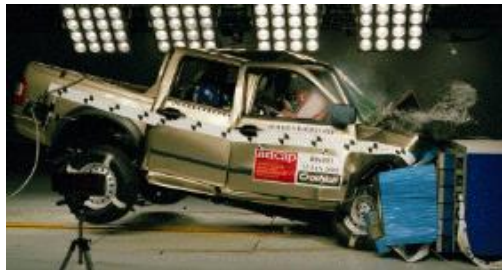
Offset crash test at 64km/hr
