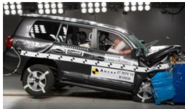
Frontal offset test at 64 km/h
