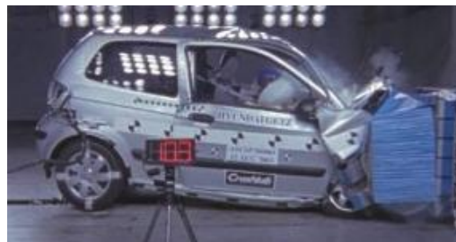
Offset crash test at 64km/hr
