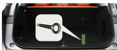
Towing hook storage location
