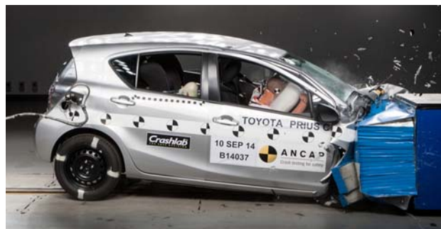
Frontal offset test at 64 km/h
