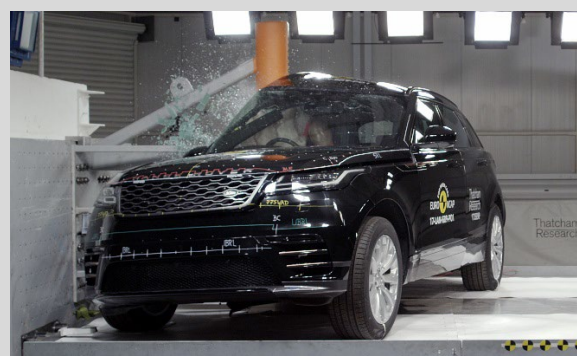
Oblique pole test at 32km/h
