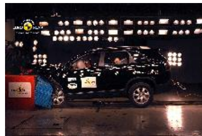
Offset crash test at 64km/hr
