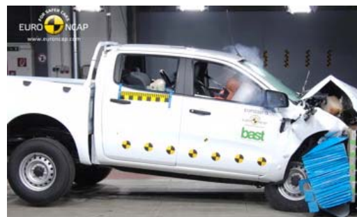
Offset crash test at 64km/h
