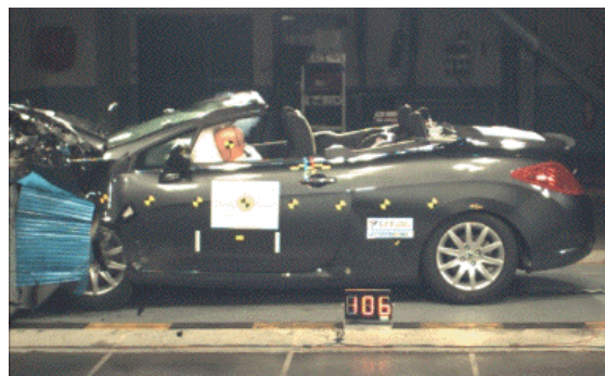
Offset crash test at 64km/h
