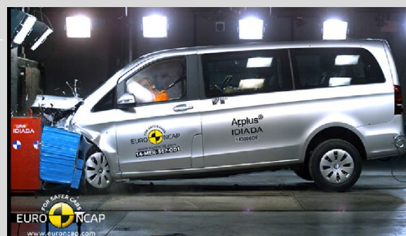
Frontal offset test at 56km/h (Mercedes-Benz V-Class)
