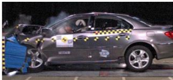
Offset crash test at 64km/hr
