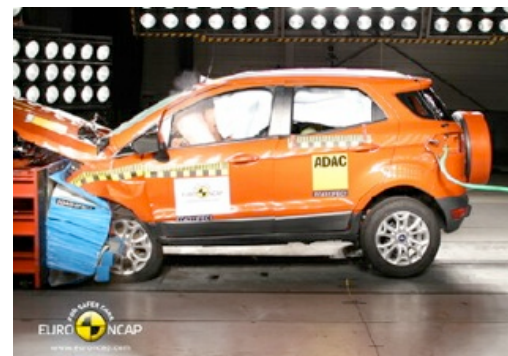
Frontal offset test at 64 km/h (Euro CAP)
