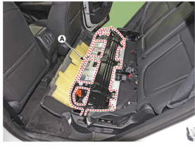
There is inlet/outlet duct and HEV battery system.
