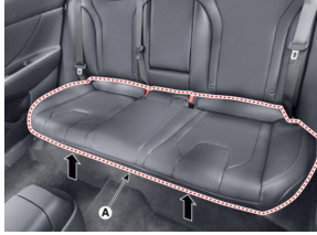
Remove the rear seat cushion assembly (A).
