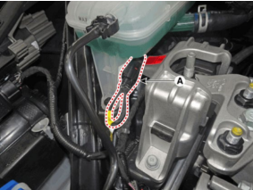
Disconnect the service interlock connector (A).
