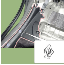
Remove the rear door scuff trim fastener (A).
