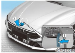
Raise the hood slightly, push the secondary latch up (1) inside of the hood center and lift the hood (2)
