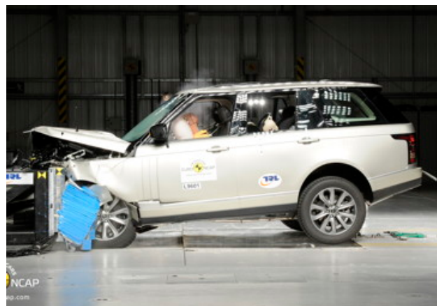
Frontal offset test at 64 km/h (Euro NCAP)
