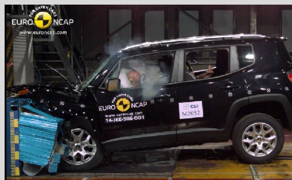
Frontal offset test at 64km/h
