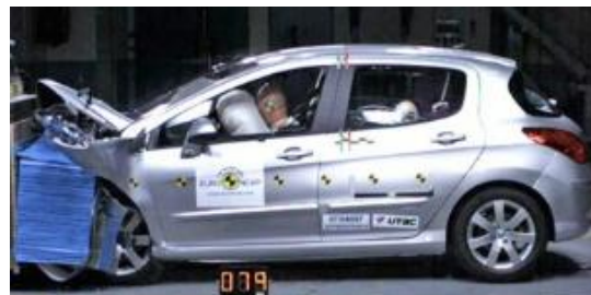
Offset crash test at 64km/hr
