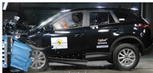
Offset crash test at 64km/h
