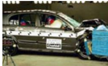
Offset crash test at 64km/hr
