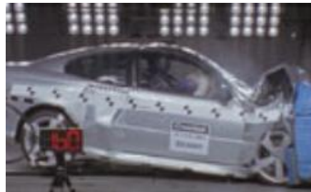
Offset crash test at 64km/hr
