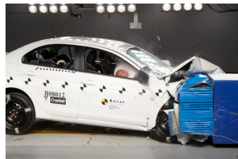
Frontal offset test at 64 km/h
