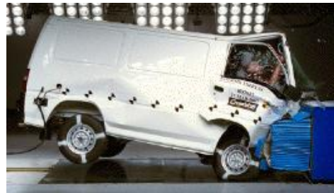
Offset crash test at 64km/hr
